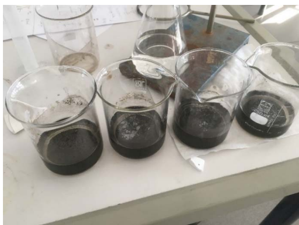
Figure 4: precipitated mixture of \text{Na}_2\text{S} and \text{Pb}(\text{NO}_3)_2 black solid is PbS.
