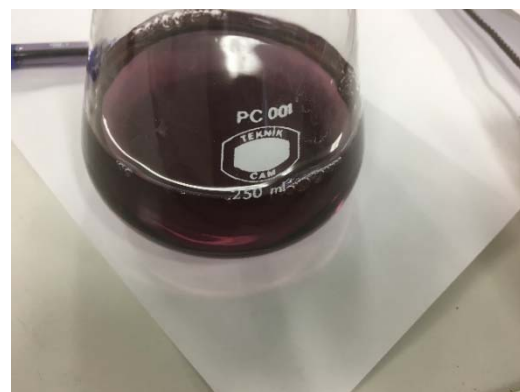
Figure 10: Mixture after titration with \text{ZnSO}_4 coloured Claret-Red.
