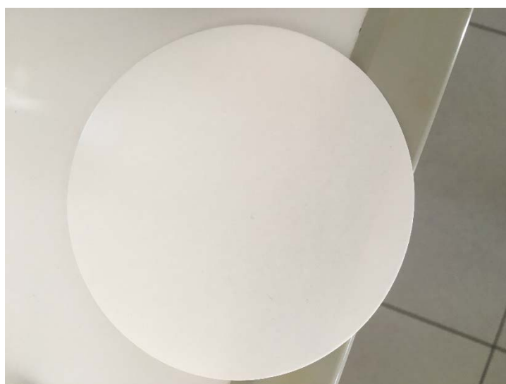
Figure 2: A filter paper used in the first method: Gravimetric method. (Xinxing)
