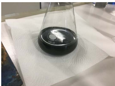
Figure 9: Mixture before titration with \text{ZnSO}_4 coloured Navy-Blue.
