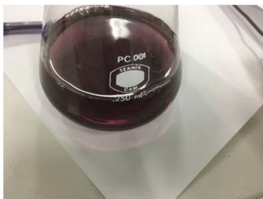
Figure 6: Resulting mixture of Complexometric Back Titration method, coloured: Claret-red
