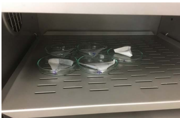
Figure 7: Filter paper in the oven to evaporate any leftover water.
