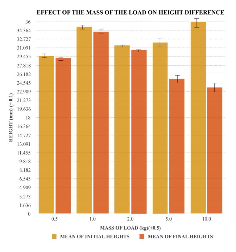
**GRAPH2:** shows how the mean of height differences differentiate with the effect of the masses of the loads and error bars which are drawn by using standard error.
