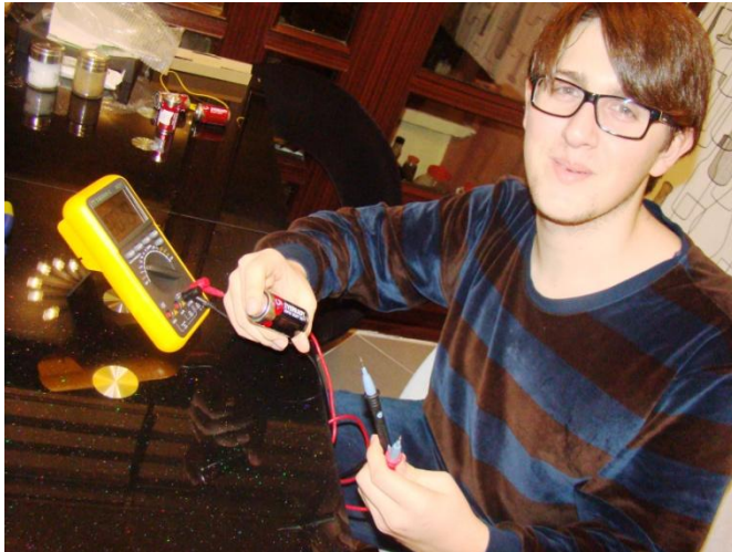
Figure 5: Shows the data collection method for electromotive force of batteries with multi-meter.
