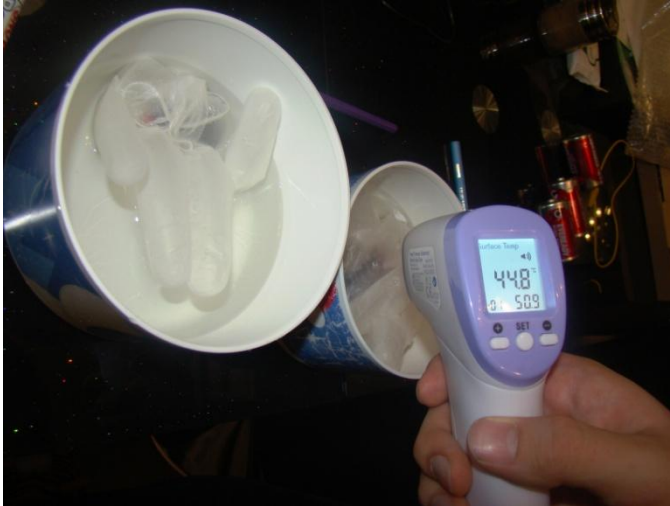
Figure 4: Shows the data collection of temperature values with using digital infrared thermometer. Batteries are in a surgical glove bag and they are In hot water.
