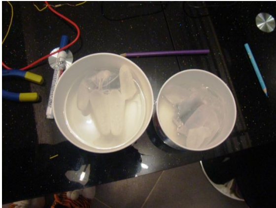
Figure 6: Shows the heating process of the battery to change the temperature. The battery is in a surgical glove to prevent the contact with water in case of possible damages to battery. The water is boiling water to increase the temperature of battery.
