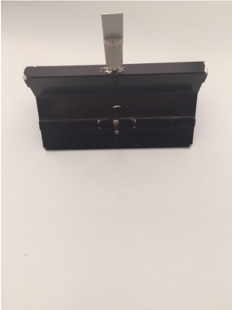
Figure 3: Glider (Total length 12.5 cm, flag length 1.0 cm)
