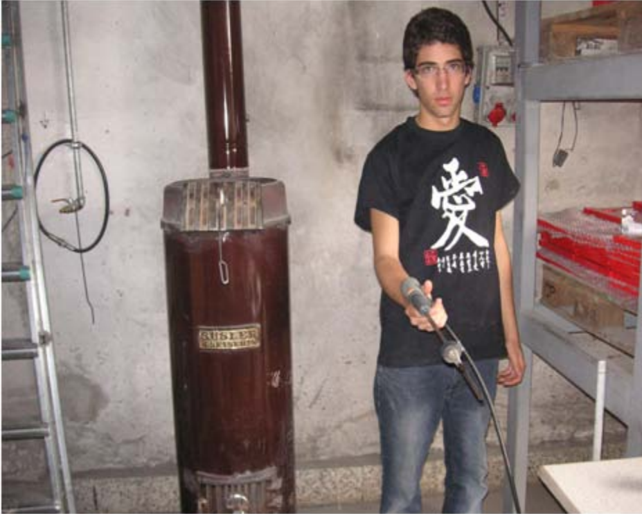
Picture 3: Measurement of the CO levels in air with one-meter distance to the stove.
