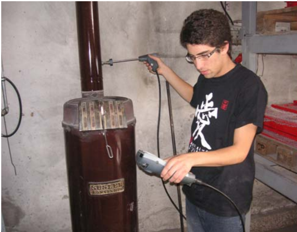
Picture 4: Measurement of the CO level in the stove interior.
