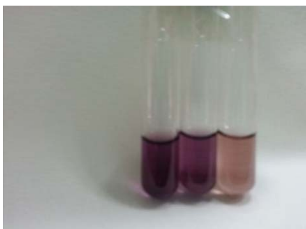
Picture 3: 3 different concentration of quercetin solutions for DPPH activity measurement
