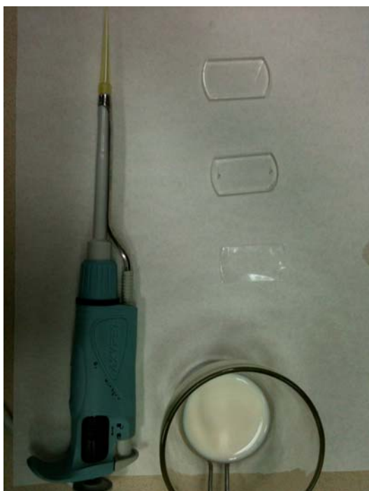
Figure 5: Micropipette, CaF 2 plates, stabilizer and milk in the glass vessel
