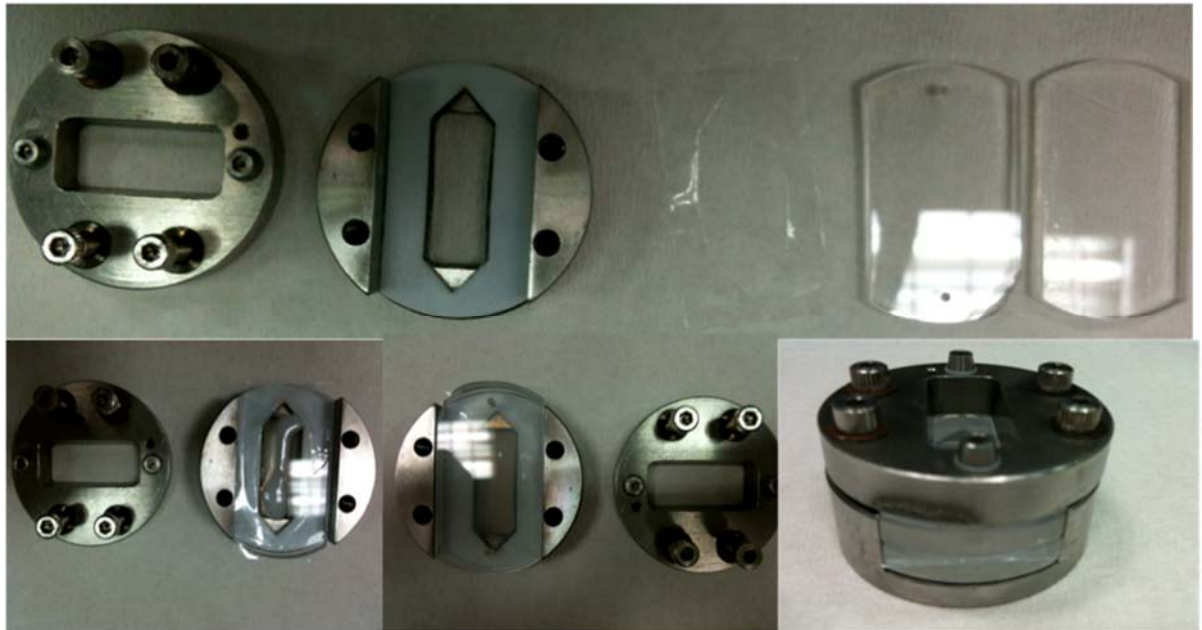
Figure 1: Process of preparing samples for FTIR
