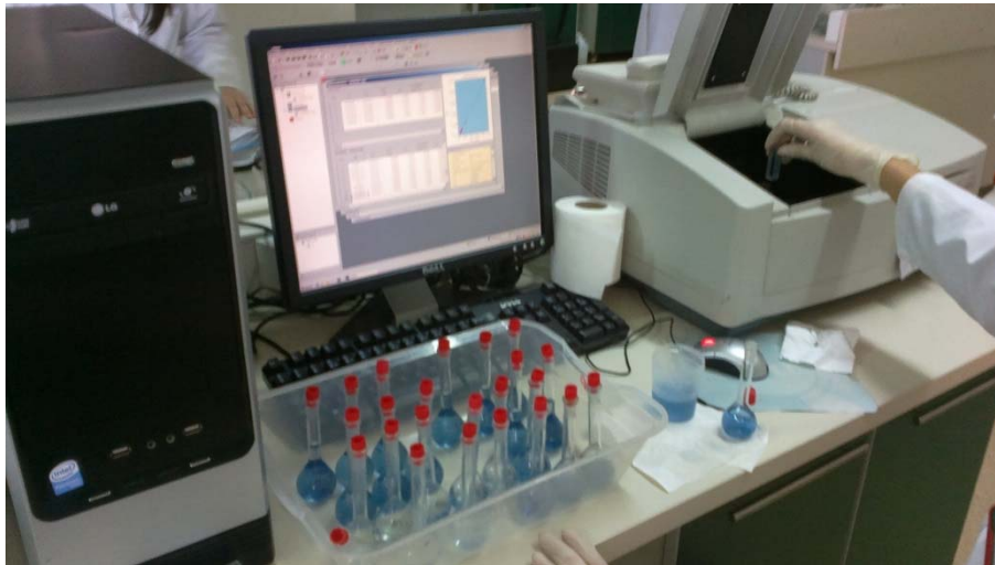
Figure 4, the detection of ascorbic acid content by using UV spectrophotometry .
