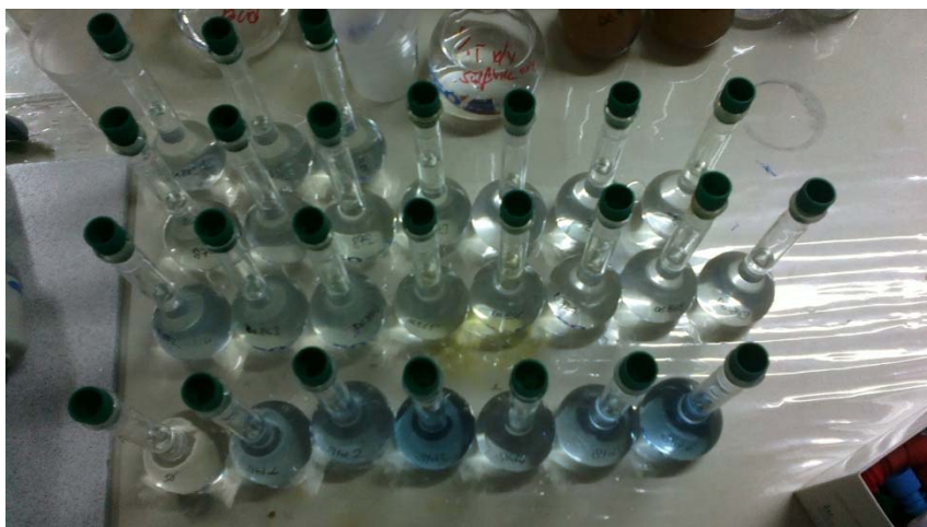
Figure 3, the balloon joji tubes of the 5 temperature groups, filled with lemon juice, water and color forming chemicals.
