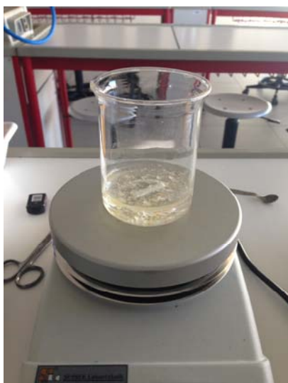
Fig6. Hexane-1,6-diamine dissolving in the water
