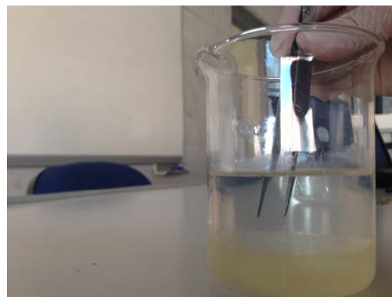
F,g8: Layer between the hexane-1,6-diamine and sebacoyl chloride solutions
