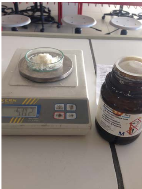
Fig5. Hexane-1,6-diamine measured for the synthesis of nylon 6,10
