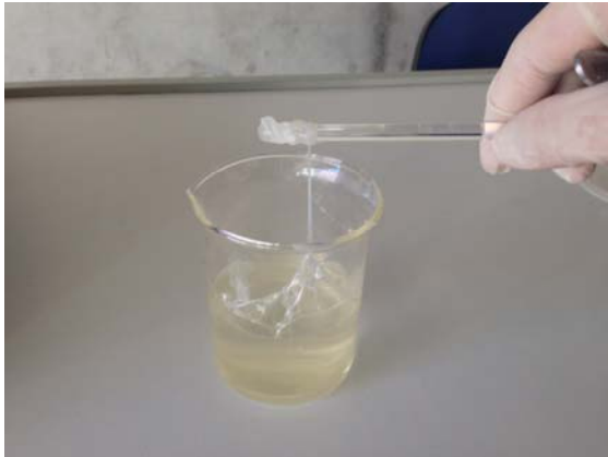
Fig9: Nylon 6,10 being extracted
