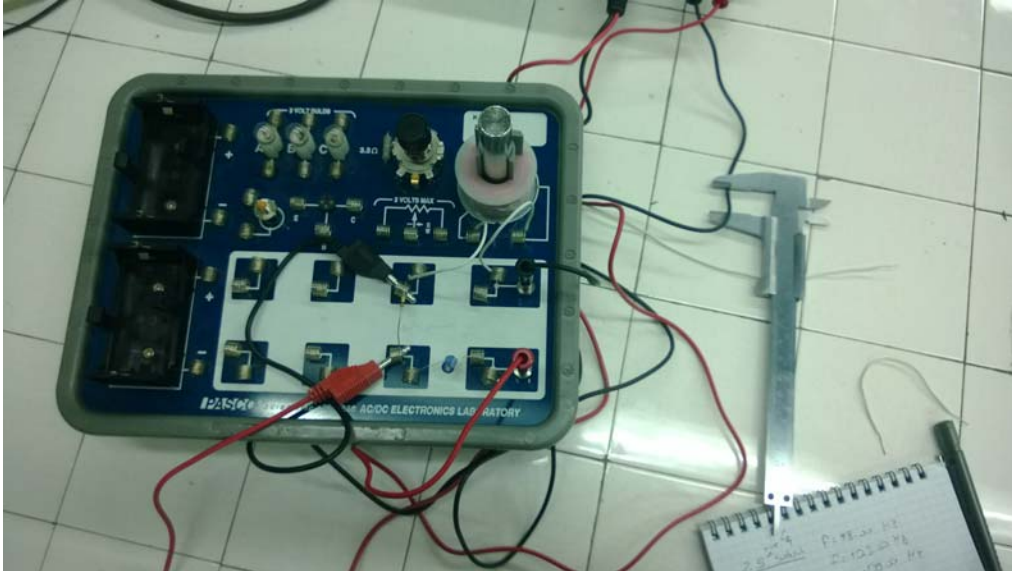
Fig 8: This figure represents the experiment apparatus. There are 2 crocodile wires (red and black), a caliper, resistor with 100 \Omega , capacitor with 100 \mu\text{F} , inductor with 8.2 \text{ mH} , iron rod (1.6 cm of radii, length of 5.0 cm), PASCO Scientific EM-8656 AC/DC Electronics Laboratory, voltage sensor and an interface.
