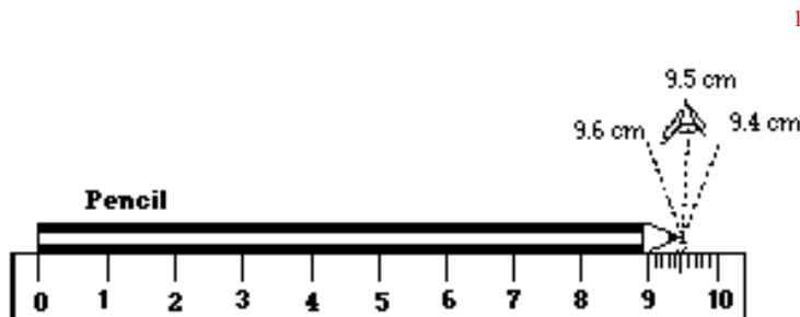
Fig 1. Example of parallax in reading the position of a point from a ruler.
