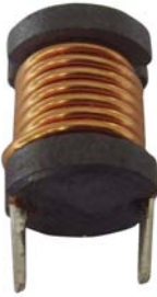
Fig 6. This is one of the inductors that is used in the experiment. 8
