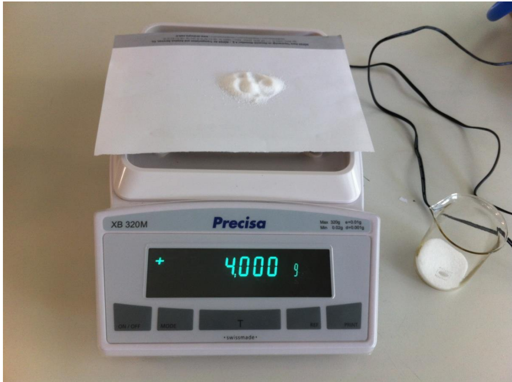
Figure 7.4.5: Example salt mass measurement at first trial of 10 cm height of water.
