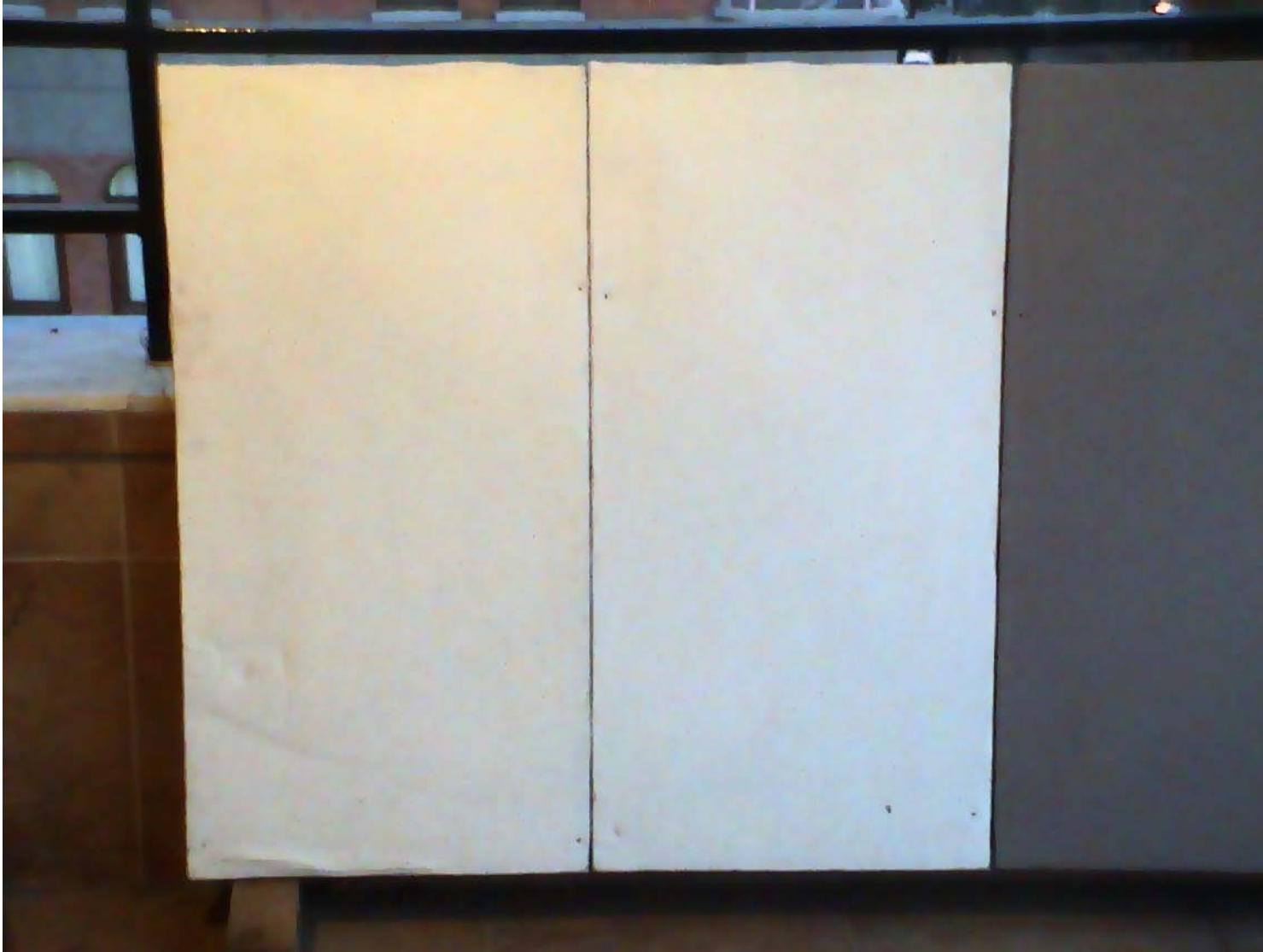
Photo 1: Showing plates number 3 and 5 coated with ZnO and TiO 2 reinforced paints respectively.
