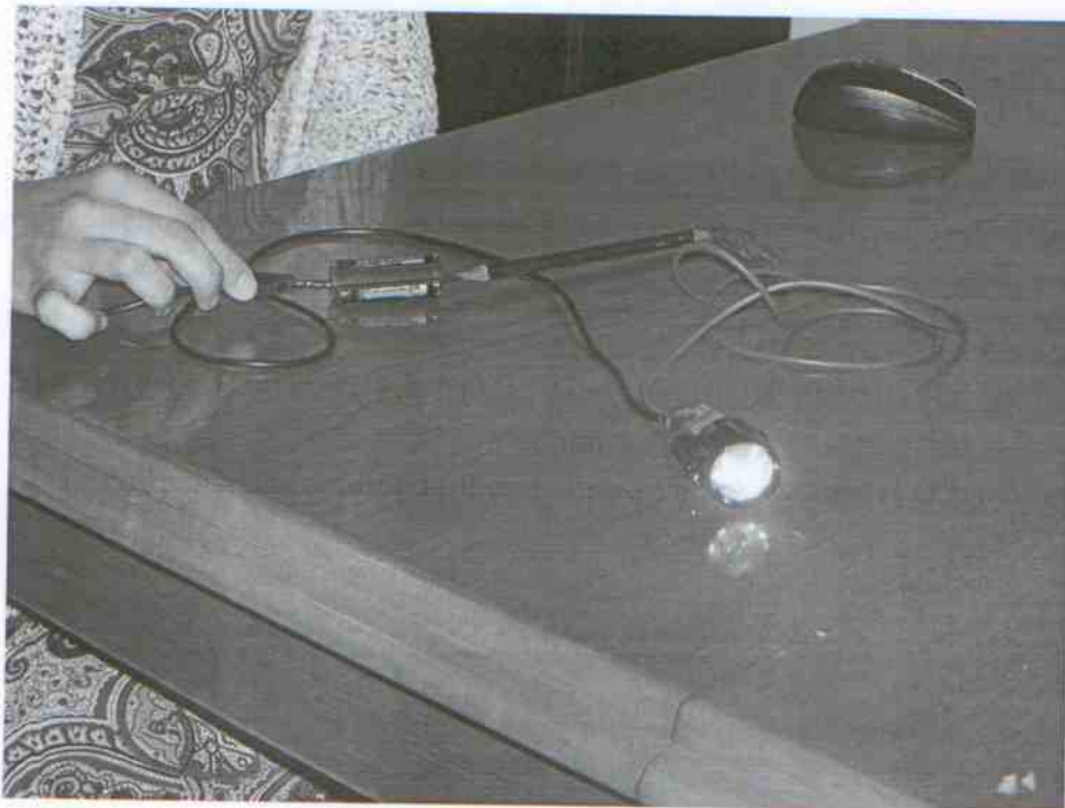
Figure 8: Shows that when a graphite pencil is used as a wire, lamp gives light, by the voltage generated from battery.
