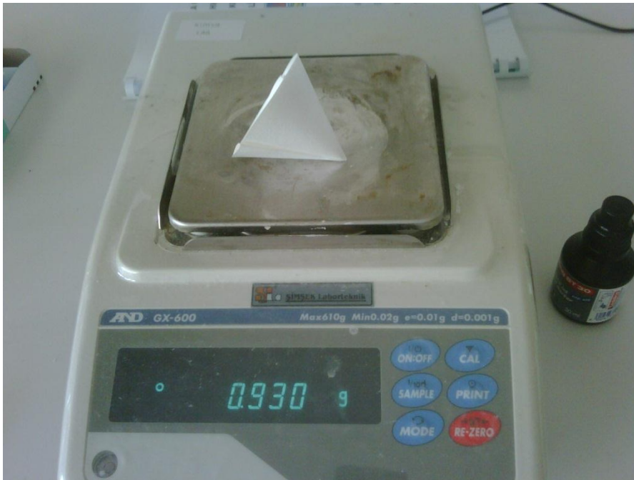
Figure 10. The filter papers were weighted after drying and the weight of the filter papers were subtracted to find the weight of \text{BaSO}_4 precipitate
