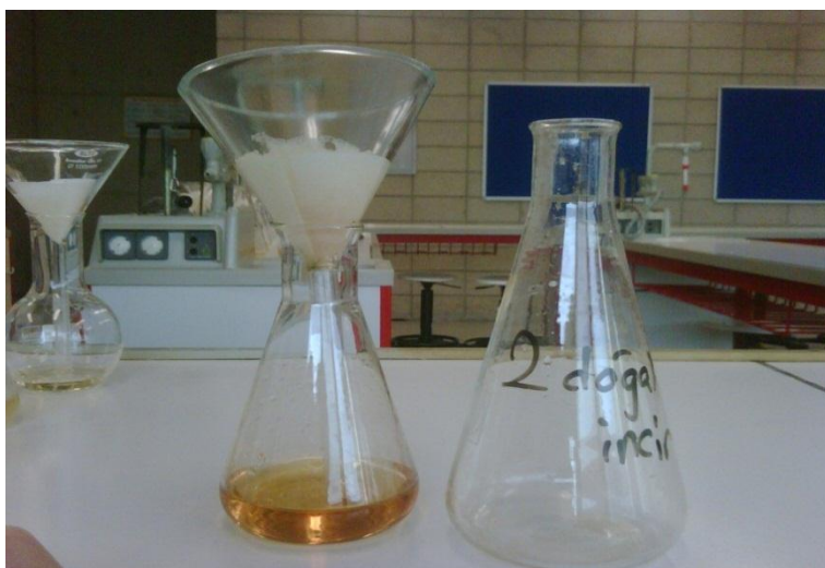
Figure 7. The solutions were filtered out so that the \text{BaSO}_4 precipitate was left on the filter
