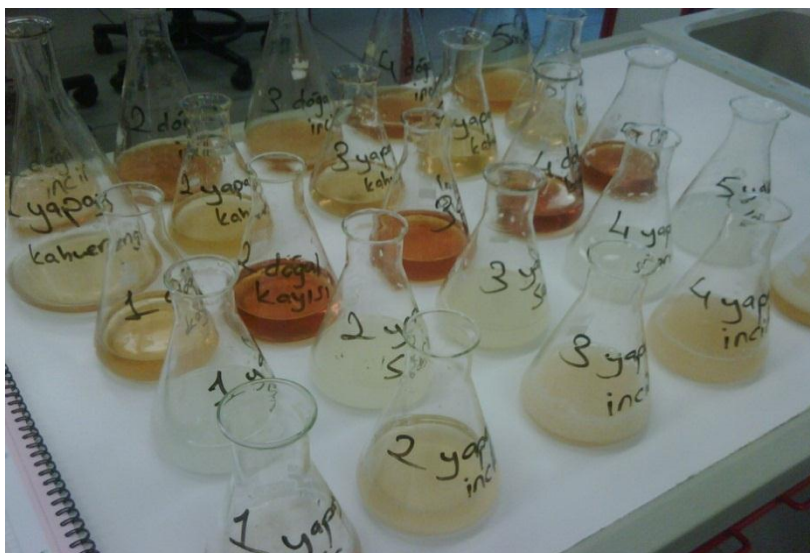
Figure 6. 30.0 \pm 0.1 mL of 3% \text{H}_2\text{O}_2 then 3-4 drops of 3M \text{BaCl}_2 were added all trials
