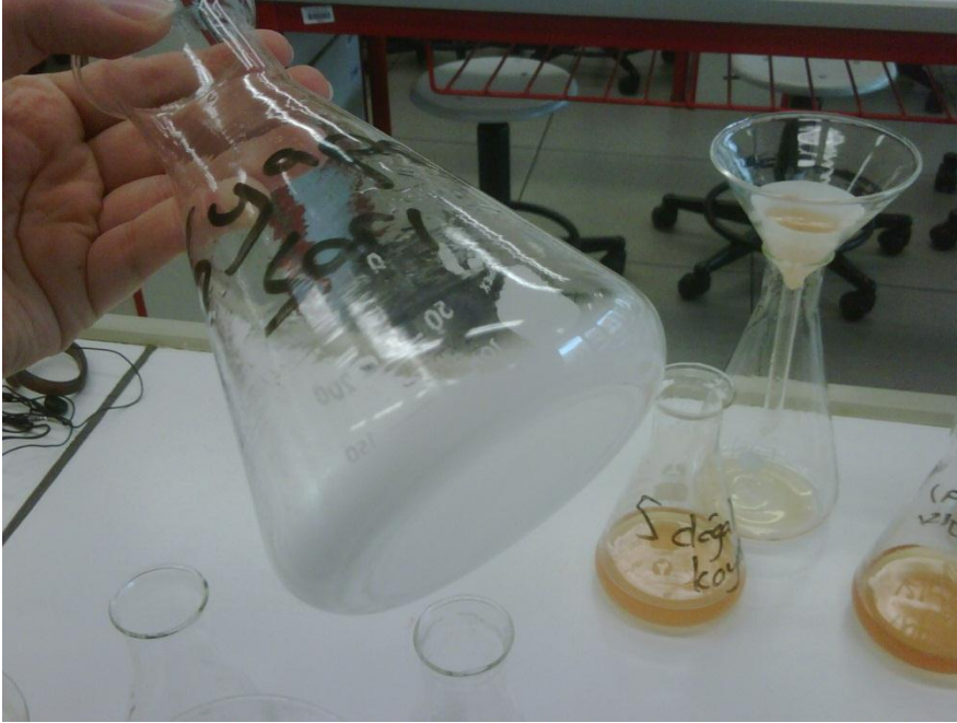
Figure 9. Most of the \text{BaSO}_4 precipitate (white) was left stuck to the bottom of the Erlenmeyer flasks in trials with artificially dried yellow apricots
