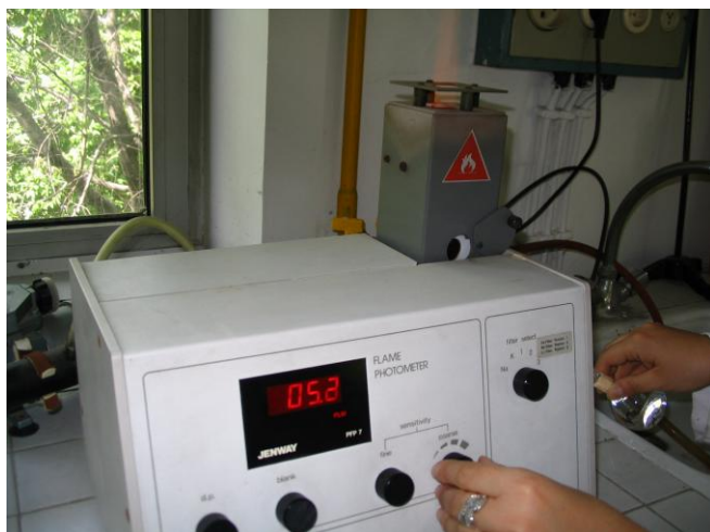
Picture 4: The flame photometer that is used in my experiment. From the colour of the flame (orange), it can be seen that sodium is being burned.
