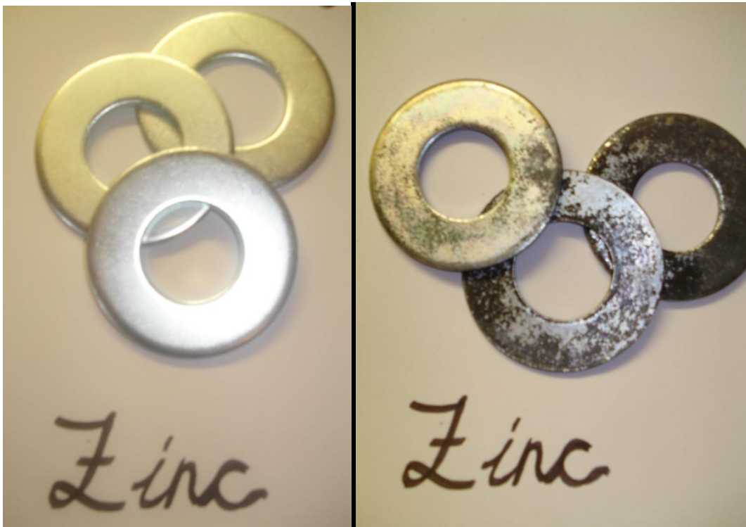
Picture 9: Pictures of zinc metals before experiment and after experiment
