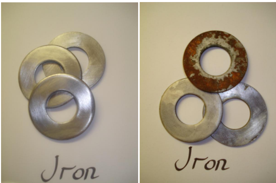
Picture 10: Pictures of iron metals before experiment and after experiment
