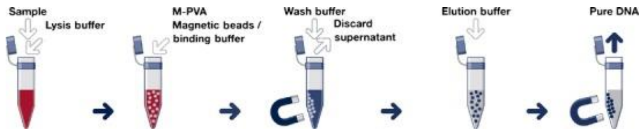
Figure 2. Schematic procedure for DNA purification by magnetic bead-based method. Retrieved from “Magnetic particles for the separation and purification of nucleic acids,” by S. Berensmeier, 2006, Applied microbiology and biotechnology , 73(3), 495–504.
