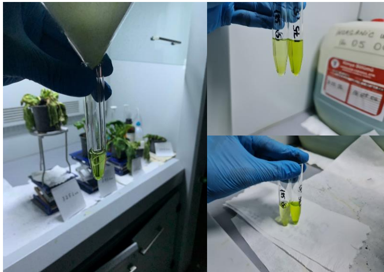
Figure 6: The extracted chlorophyll inside the test tubes with a vibrant color difference caused by the difference in chlorophyll amount
