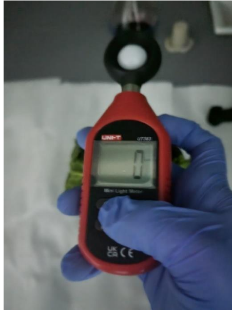
Figure 10: The Luxmeter that I used to measure the light intensity on the plants.
