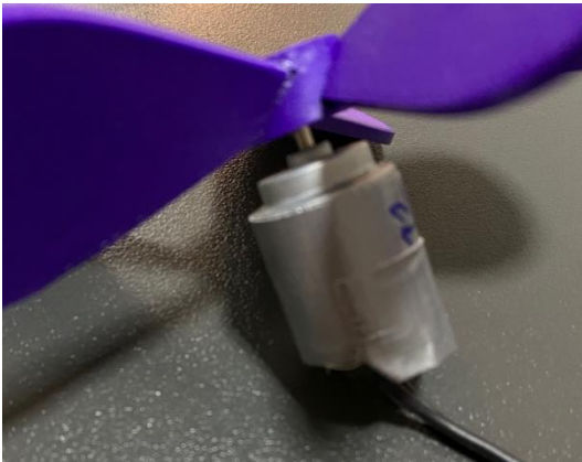
Figure 8.4: Motor and Turbine Connection
