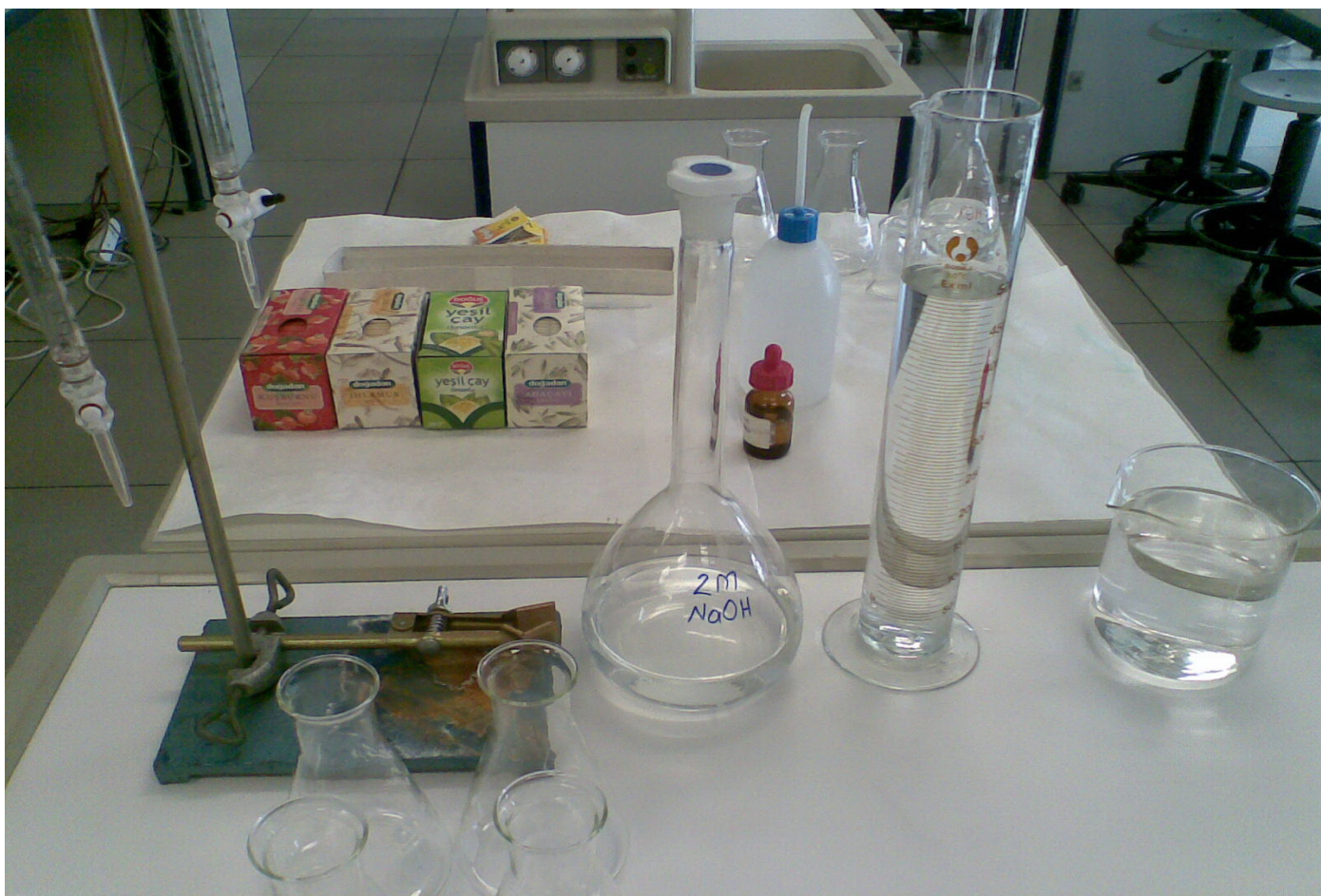
Picture 5 (above): My apparatus I used for my trials. At the left front, you see the 4 250 mL beakers. In the middle, there is 2 M NaOH. At the left of the 2 M NaOH, there are the burettes.
