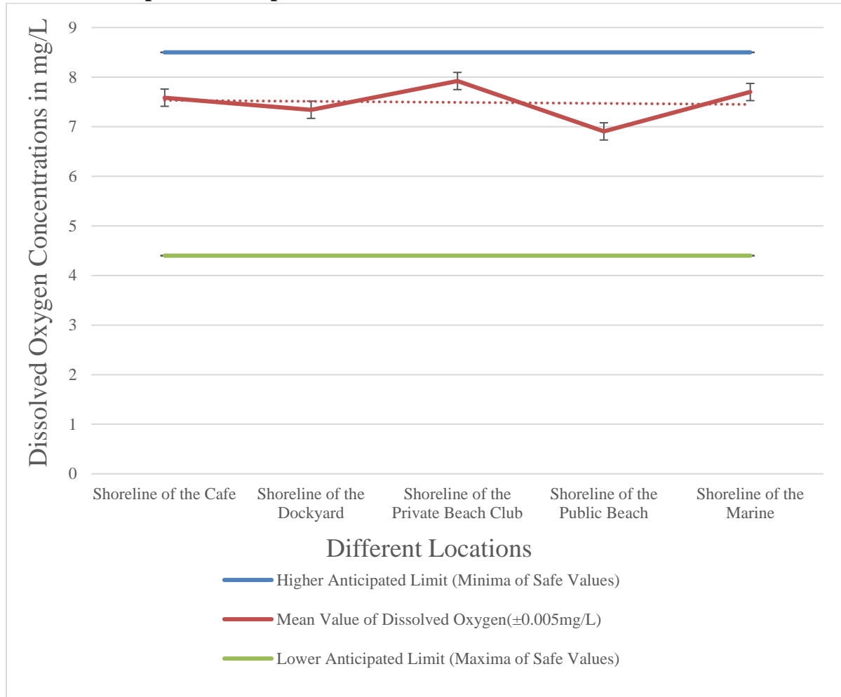
Graph 1: This line graph illustrates the relationship between different areas and their dissolved oxygen concentration in mg/L which is the research question of the assessment. As the profiling studies and decided safe limits have very low uncertainties especially compared with my measurements, they will be neglected. Upper and lower limits which were discussed previously and given in Table 1 are entertained, showing all values are healthy even in Aegean standards. Seeing a trend among different places with the help of a dotted trend line is possible in this line graph.
