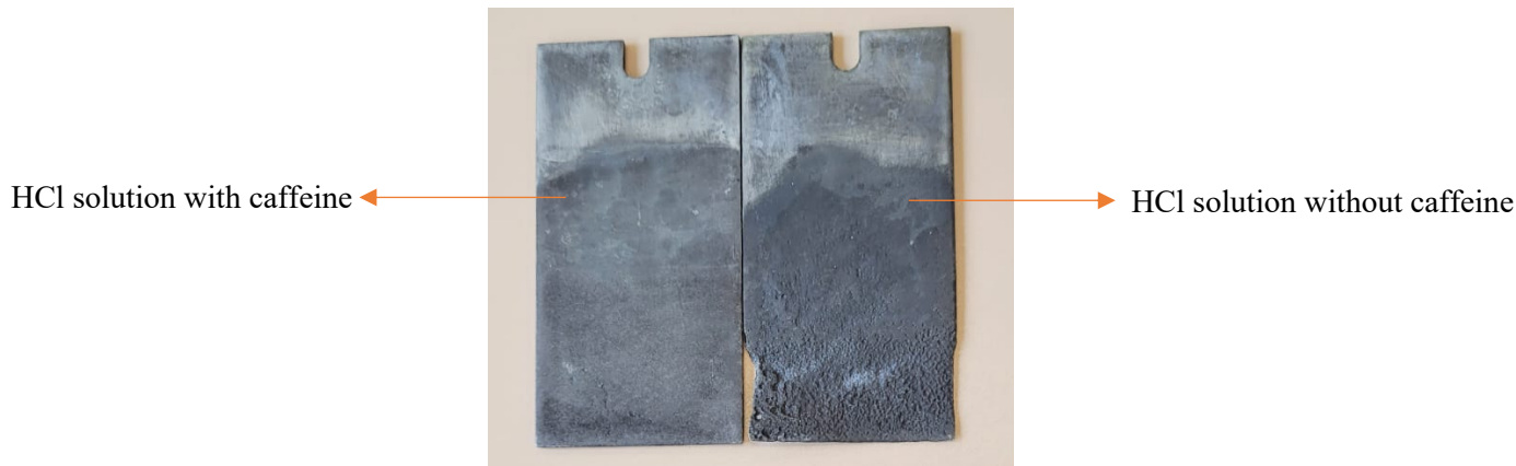
Figure 10: Zn specimens waited inside HCl solutions with (Right) and without (Left) caffeine added.
