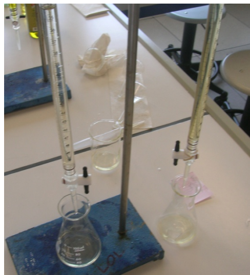
Picture 3: Burettes are shown. One of them is filled with n-propanol solution, the other one is filled with oil.
