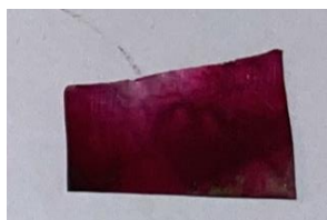
Figure 4. dyed aluminum piece anodized at V=17.1V
