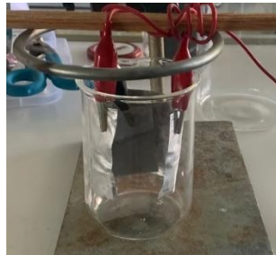
Figure 2. set up of aluminum cathode anodizing
