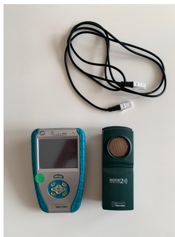
Photo 2: Motion sensor and LabQuest 1
