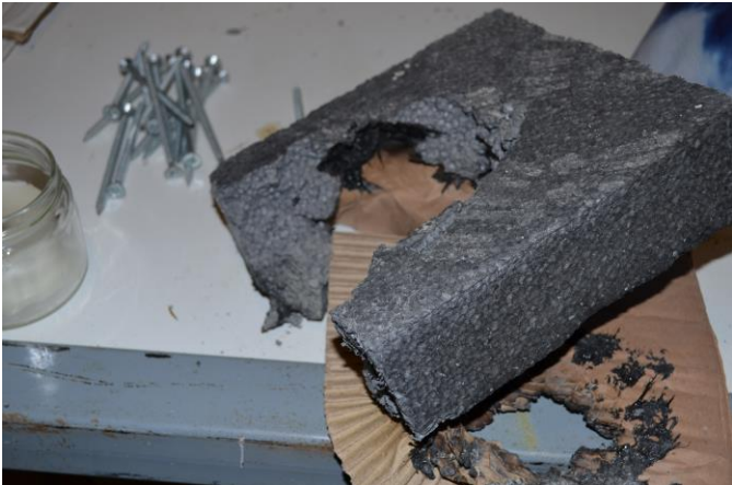
Figure 4: Photo of the melted EPS due to heat
